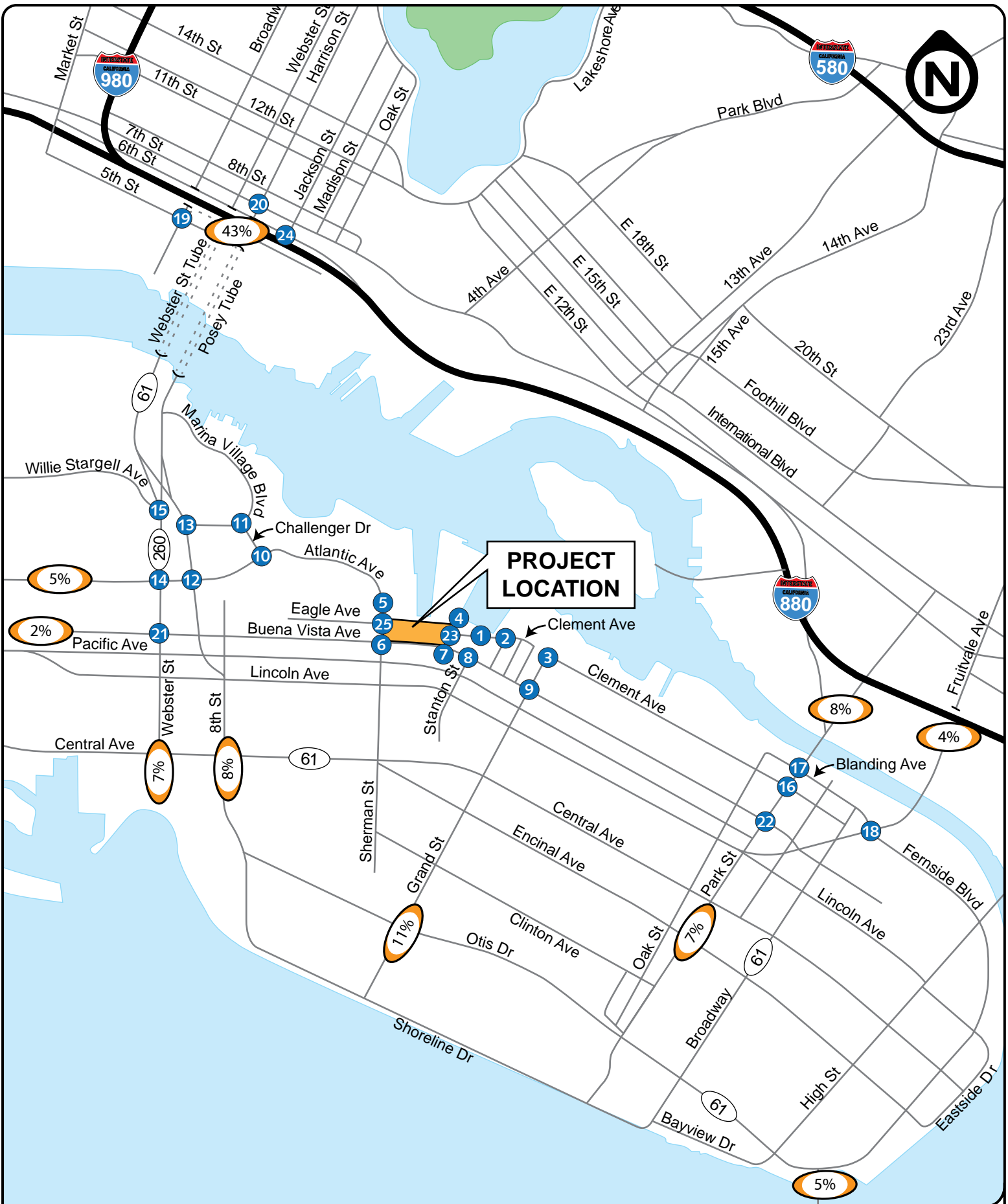
FIGURE 5 | PROJECT TRIP DISTRIBUTION TRANSPORTATION IMPACT ANALYSIS Del Monte Mixed Use Project City of Alameda
